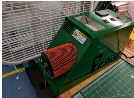
Figure 3: Filabot extruder used in the filament recycling process
