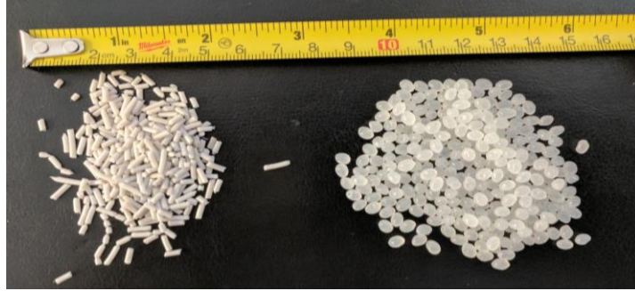
Figure 2: Filament pellets (left) vs. virgin pellets (right)
