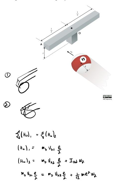
$$e = \frac{V_{A2} - V_{b2}}{V_{b_1} - V_{A1}} = 0.8 = \frac{W_{\lambda} \frac{2}{\lambda} - V_{b\lambda}}{V_{b_1}}$$
