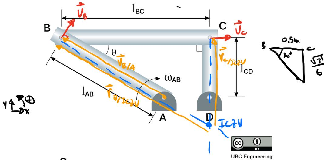
$$\begin{aligned}\vec{v}_B &= \vec{v}_A + \vec{\omega}_{AB} \times \vec{r}_{B/A} \\ &= (-5 \text{ rad/s } \hat{k}) \times (-0.4 \cos 30^\circ \hat{i} + 0.4 \sin 30^\circ \hat{j}) \\ &= 2 \cos 30^\circ \hat{j} + 2 \sin 30^\circ \hat{i} \text{ [m/s]}\end{aligned}$$
