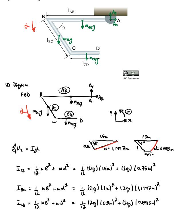
$$I_A = I_{AB} + I_{BC} + I_{CO} = 11.2758 \text{ ig m}^A = I_A$$
