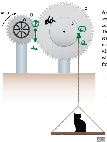
A cat has found itself stuck on a platform controlled by a gear system. A bystander attempts to save it by turning handle A at a constant 5 rad/s<sup>2</sup> in the clockwise direction.
